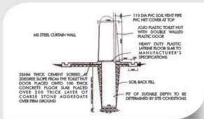
Diagram 2 - Collapsing Soil Installation
